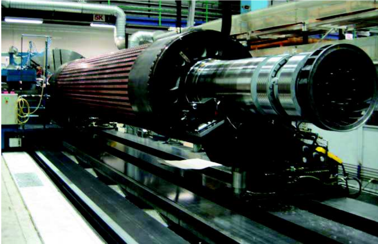
Figure 3: 110-ton rotor of 138 MVA single-phase generator
